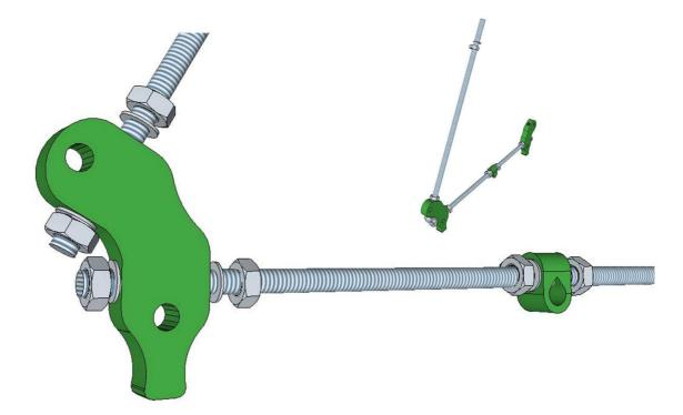
Take the third piece of threaded rod and put a nut and washer on one end. Thread the free end of the rod through the other foot and place a washer, 2 nuts and a washer on the other end as shown. Now thread that end through the top vertex and fix it in place with a washer and nut.
